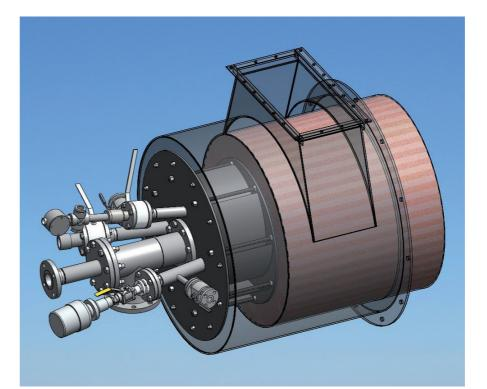
Thus, a large portion of the hot flue gas tending to exit the combustor is drawn into the center core where it is recirculated toward the fuel tip nozzles.
