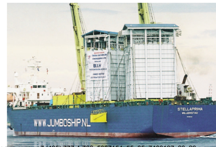
Shipment of complete reformer heaters with burner already installed
